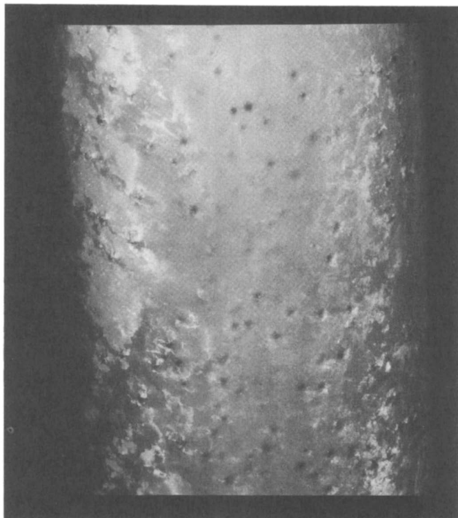
Figure 6. Close-up photograph of D1B76 ( d=109 nm, \phi=0.1 ) suspension in the presence of the Bio-Rad resins. Outside diameter of the vessel is 15 mm.
